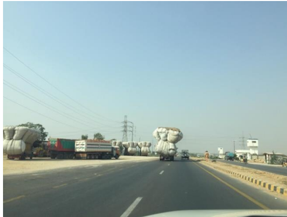
Figure 28: Improperly loaded trucks
